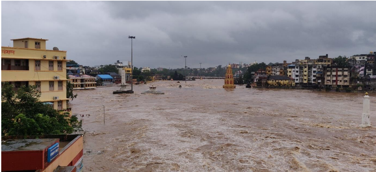
Fig. 6. A view of UGR upstream of Sarkarwada (See location in Fig. 1) on 5 th August 2019 (a day after the August 2019 flood). Width of flow 128 m and depth of flow 9.71 m (Photograph taken from Holkar/Victoria Bridge, Nashik).
