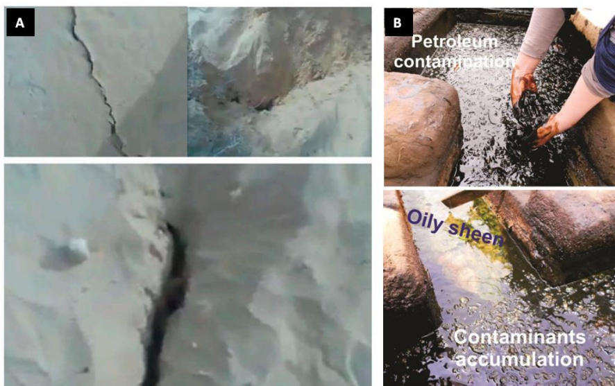
Fig. 4. Observed degradation issues: A. Land subsidence (Hamed et al. 2014a); B. Petroleum contamination (Besser, Hamed 2019).
